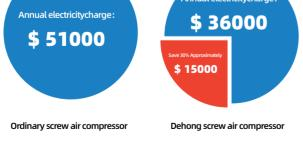
Calculation conditions: Operation time :8000 hours/year, electricity cost 0.1USD/KW/H, average load 84%
